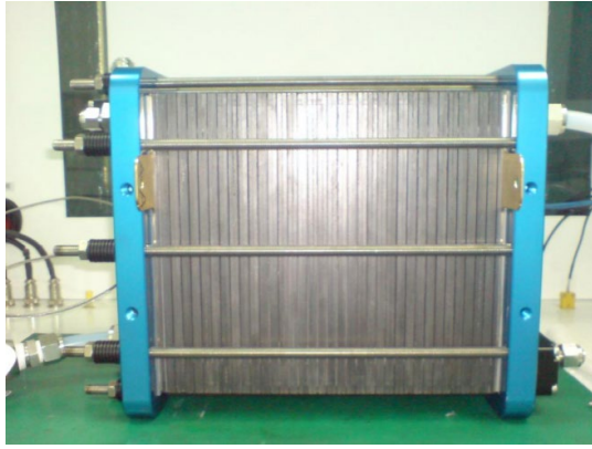
Figure 11. Fuel cell stack (FCE-1.2kW-07) of Fucell Company
